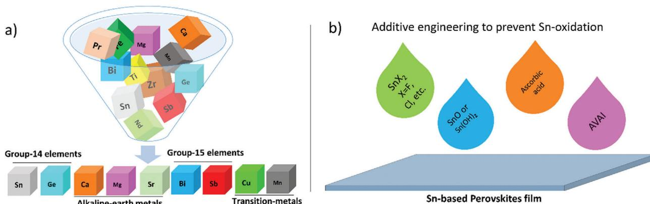
**Figure 3.** a) Possible non- or less-toxic alternatives to replace Pb (filtered from the periodic table) in the organometal halide perovskite framework. b) Additive engineering to maintain Sn in its bivalent state and improve the film morphology. Various species are shown which are utilized into the precursor solution of the Sn-based perovskites.
