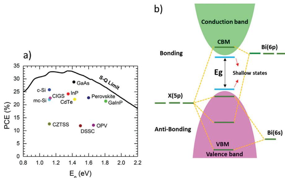
**Figure 5.** a) Maximum PCE (Shockley–Queisser limit) for a solar-cell operated under AM 1.5G illumination at 298.15 K, as a function of the energy bandgap. Reproduced with permission.<sup>[54]</sup> Copyright 2018, American Chemical Society. b) Electronic band structure of the Bi-based perovskites and formation of shallow states, indicating their defect tolerance nature.
