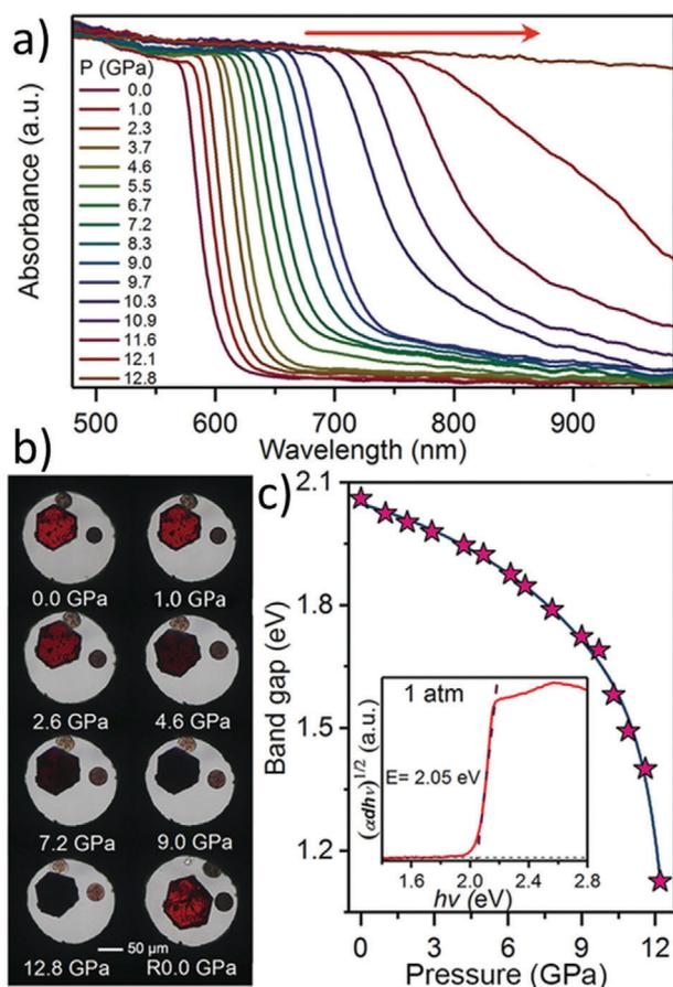
**Figure 18.** a) Optical absorption spectra of CBI under high applied pressure. b) Optical images of CBI in a diamond anvil cell (DAC) upon compression. c) Bandgap evolutions of CBI under high pressure. The inset of the figure shows a Tauc plot for CBI at 1 atm. Reproduced with permission.<sup>[147]</sup> Copyrights 2018, Wiley-VCH.
